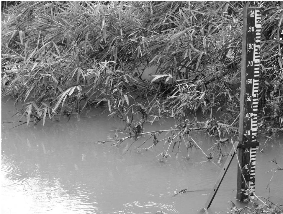
Figure 10: One of the sampling site with Water level indicator
